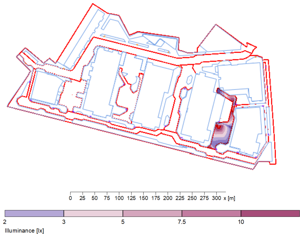
Figure 5.3.5 - Illumination Levels to Accessible routes
