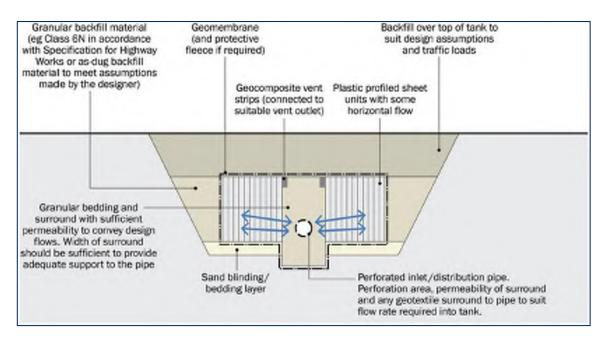
Figure 3.12 - Typical Section of Geocellular System (CIRIA C753)
