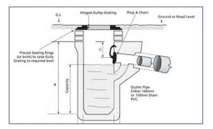
Figure 3.10 - Trapped Road Gully (Typical Detail)
