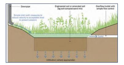
Figure 3.7 – Rain Garden (Typical Detail)
