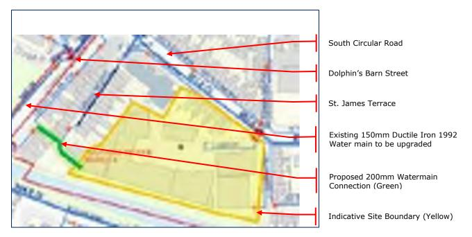
Figure 5.2 – Water Connection (Confirmation of Feasibility)
