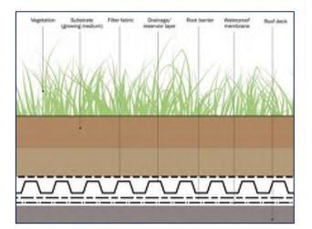
Figure 3.6 – Typical Green Roof Build-up
