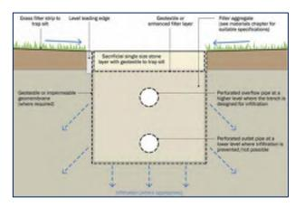
Figure 3.9 – Filter Trench (Typical Detail)
