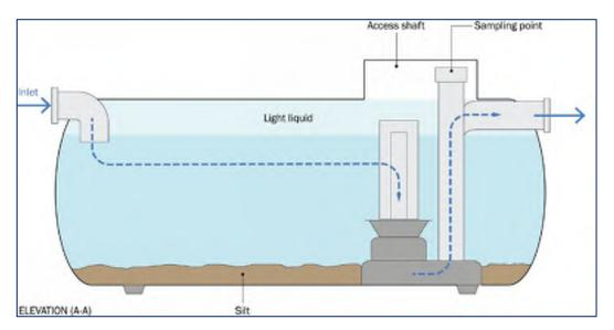
Figure 3.14 - Typical Section Detail of Fuel Separator (CIRIA C753)
